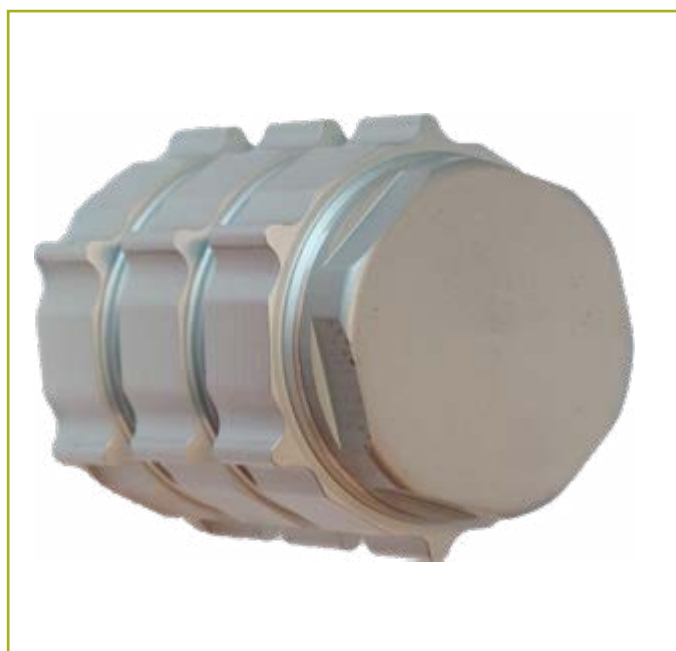
Filter holder containing filter pack, to be mounted in the funnel.
