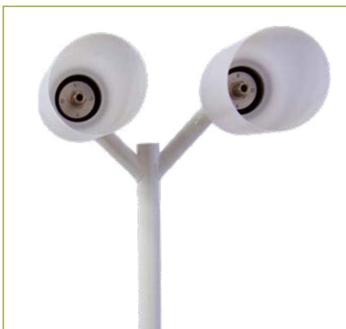
Funnels, to protect the filter holder containing the filter pack.
