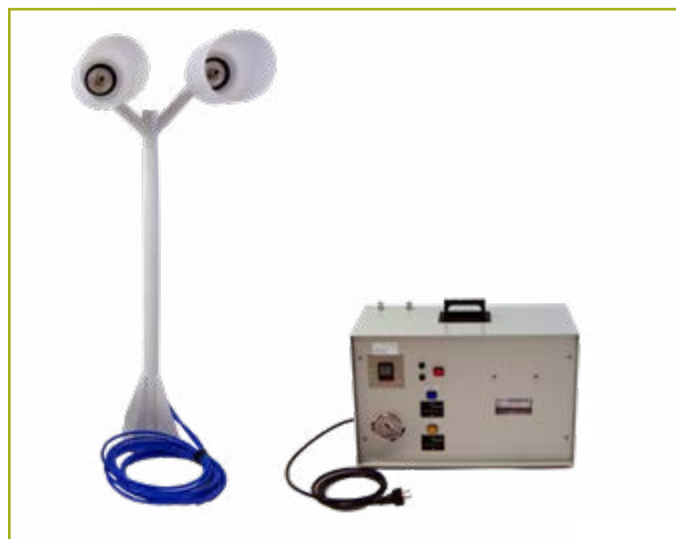
EK Sequential Air Sampler – funnels with control unit.
